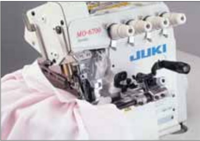
● For gathering MO-6714S-BE6-327/S162 (S162: Swing-type gathering device)
