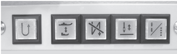
Simple setting for alternating presser foot movement
